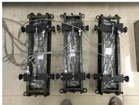
Figure 4 UHPC autogenous shrinkage testing device
