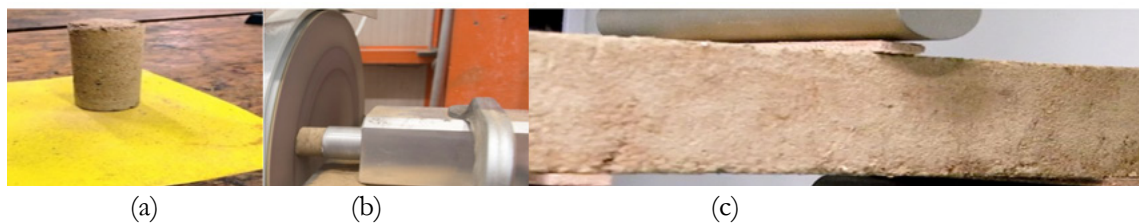
Figure 4: Sanding paper (a) and machine (b) used for rectification purposes and wooden strip interposition between steel rolls in a three point bending test (c) [20], [21]
