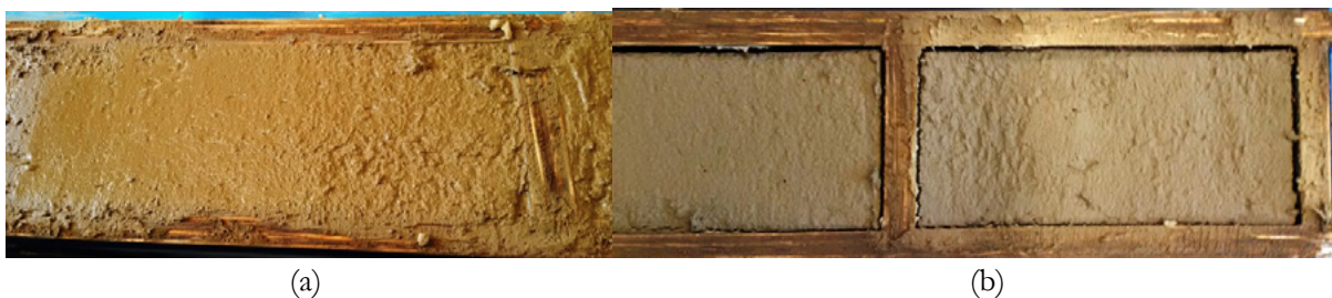
Figure 5: Picture of mortar just casted(a) and after five days since pouring(b): volumetric shrinkage of about 18%[22]
