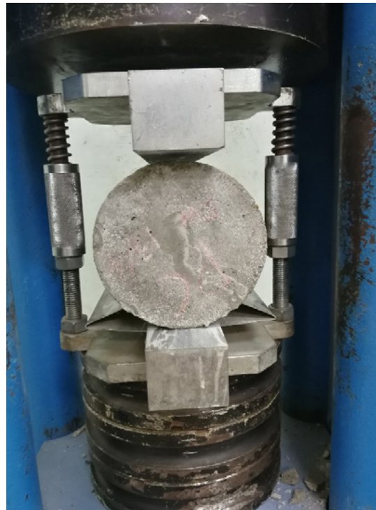
Figure 2: A cylinder specimen under splitting tensile strength test.
