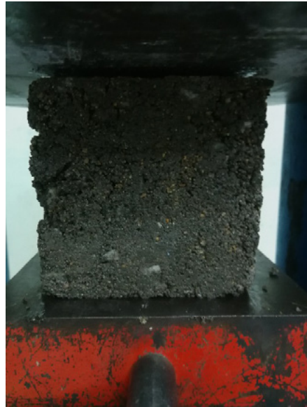
Figure 1: A cubic specimen under compressive strength test.
