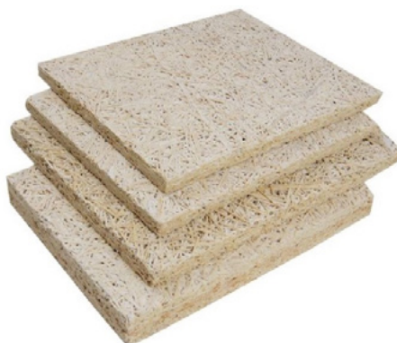
Figure 2: Wood wool cement board (WWCB) manufactured with spruce wool
