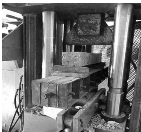
Figure 3: Flexural testing of RCA beam specimens on UTM
