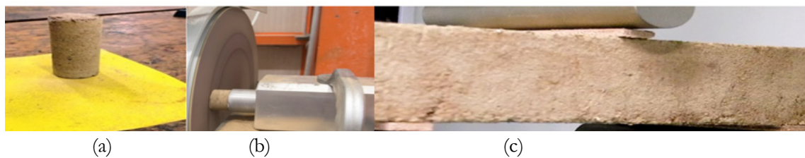
Figure 4: Sanding paper (a) and machine (b) used for rectification purposes and wooden strip interposition between steel rolls in a three point bending test (c) [20], [21]
