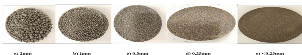
Figure 1: Morphology of air granulated slag sieved into different fractions. The smaller fractions c) 0,5mm d) 0,25mm and e) <0,25mm have contamination that can be observed with the naked eye.
