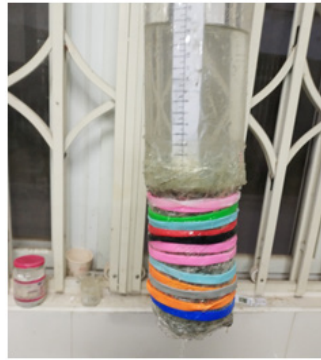
Figure 2: The apparatus for permeability test.
