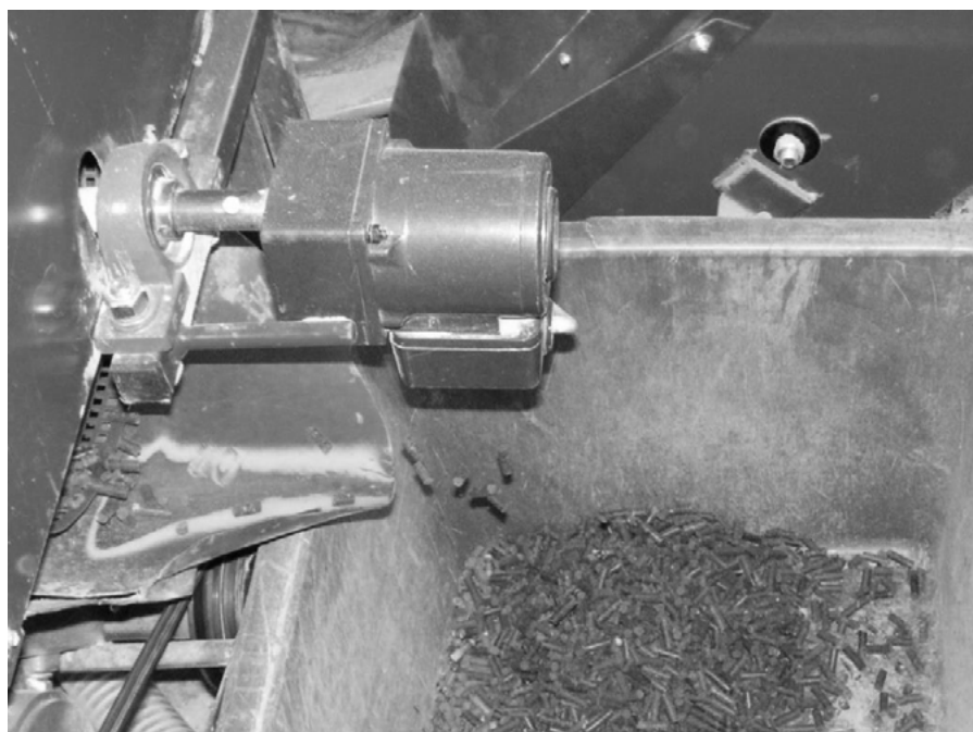
Figure 1: Preparation of pellets from MBM in the granulator line MGL 200
