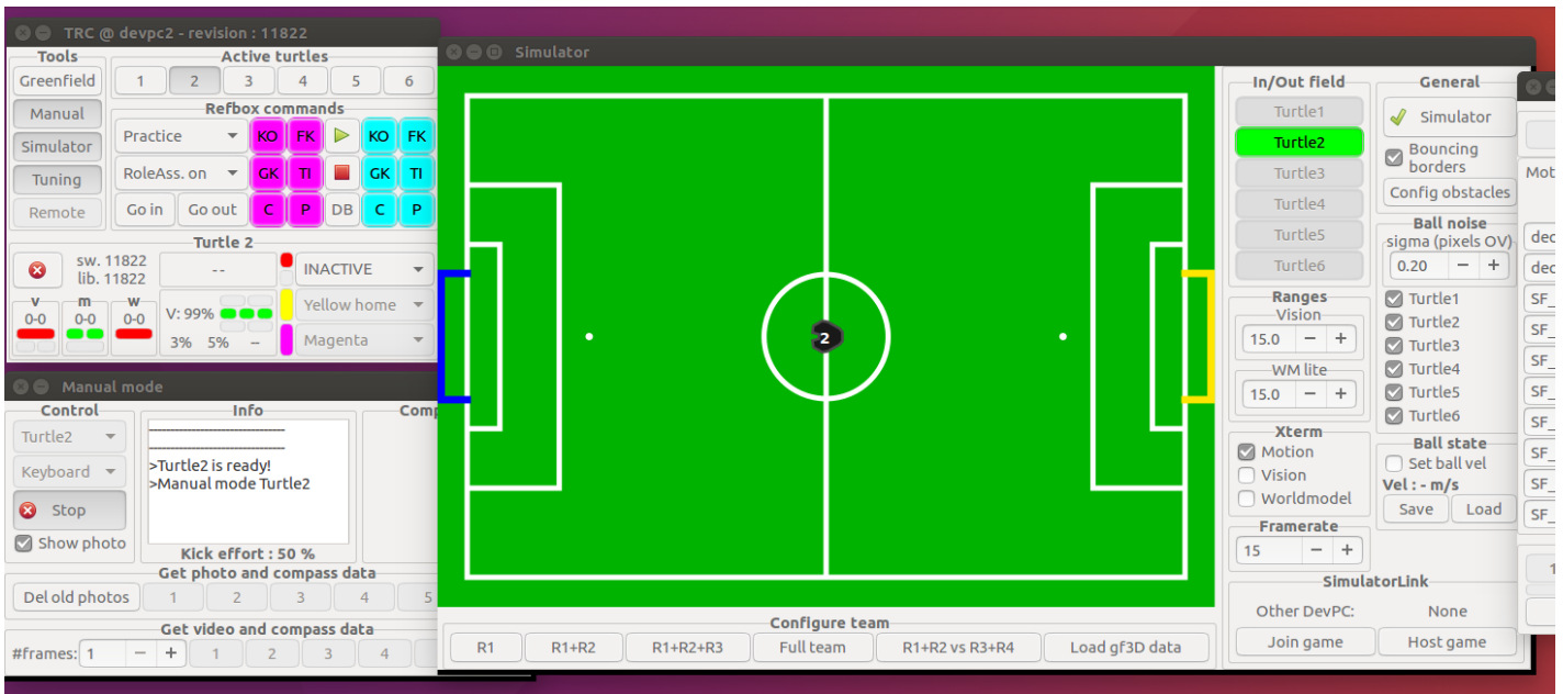
Figure 7.4: This screenshot from the eNB computer shows the Turtle Remote Control (Top left), the Manual Control window (Bottom left) and the Simulator view on the right. On the TRC, Turtle 2 is chosen and the values v , m , w show which executables are running. The green LEDs under m shows that Motion and Strategy executables are communicating. The info tab on the Manual mode window shows that Turtle is ready, which means that a connection is established between the Turtle software on the UE and the eNB.
