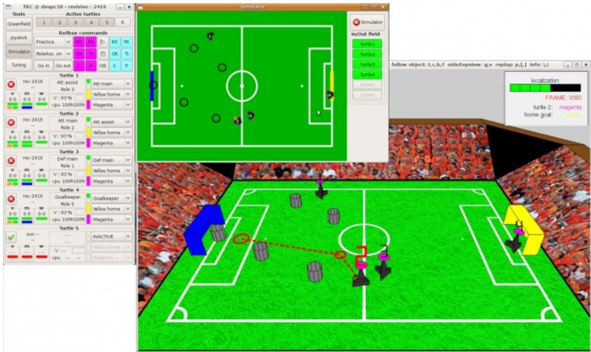
Figure 6.5: This figure is a screenshot of the Turtle Simulator in action. On the left is the TRC GUI, the image on the top describes the simulator used in this project and the image on the bottom describes the Greenfield simulator that provides a 3D simulation of the gameplay with additional information such as the status of the robots and the ball position. The Turtle simulator is able to show both the Tech United robots as well as opponent robots and the ball. In this project, only one robot was visualized by using the shared sensor data. [7]
