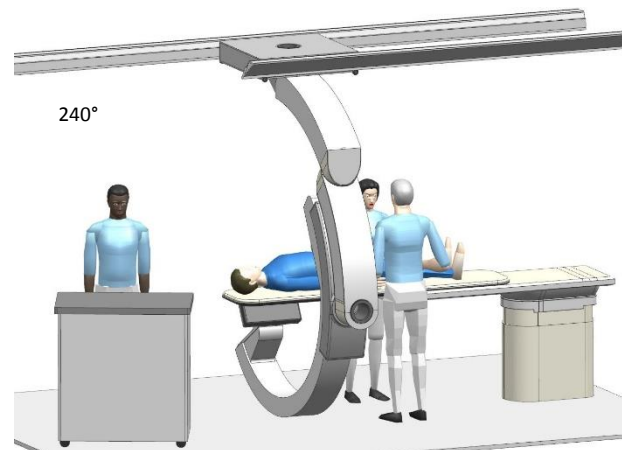
Figure 3. System 1: additional rotational joint allows for a 300° extended 'roll' scan ( -60^\circ to +240^\circ ).
