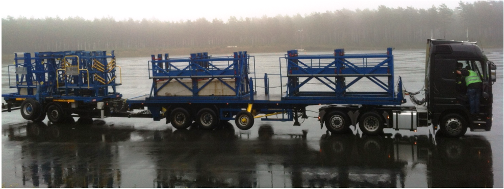
Figure 6.2: Vehicle combination used in reversing tests.
