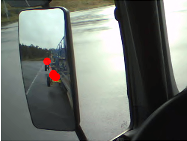
Figure 6.5: Continuous gazing between the outriggers to estimate the orientation of the last vehicle unit, as observed on majority of drivers
