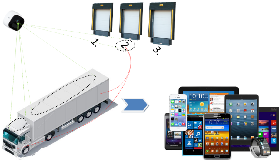
Figure 7.15: Concept of Driver Support Functionality using the vision based localisation, smart phone as HMI.
