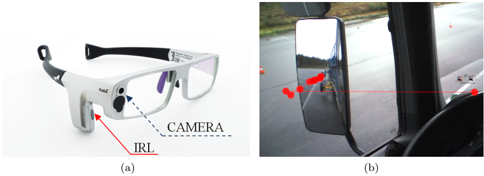
Figure 6.3: (a) Tobii eye-tracking glasses (b) Illustration of the drivers view with the gaze point.
