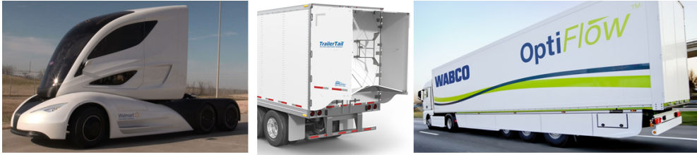
Figure 4.11: Aerodynamic drag reducing components (from left to right): Aerodynamic and prolonged cabin [132], Foldable boat tail [118], Side skirts [131].
