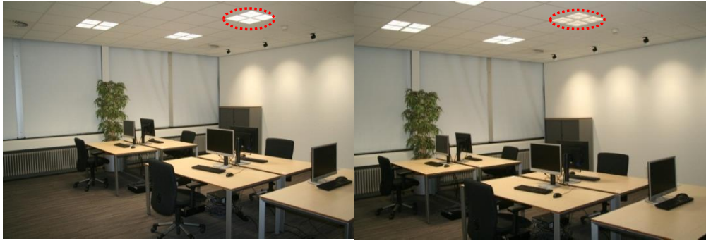
Figure 41. Impression of the room with luminaire L4 in an 'occupied' state with a horizontal desk illuminance of 543 lx at desk 4 (left) and a 'vacant' state with a horizontal desk illuminance of 310-345 lx at desk 4 (right).
