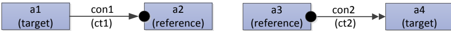
Figure 5.7: Two behavioral cardinality constraints: con1 and con2 . Inspired by Declare , the dot indicates the reference activity . The target activity is on the other side that has no dot. The constraint type is represented by the arrows.
