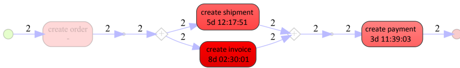
Figure 8.28: Analyzing the performance based on the log in Figure 8.24 with Inductive visual Miner (setting parameters “activities” as 1 and “paths” as 0.2).
