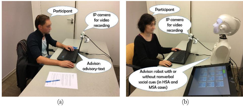
Figure 4.2: Experimental set ups (a) Low Social Agency (LSA) (b) Medium Social Agency (MSA) and High Social Agency (HSA).
