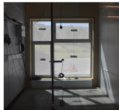
► Fig. 3: View of the inside of one of the twin test cells.
