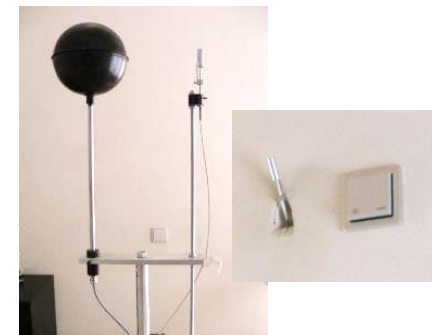
► Fig. 4: Indoor thermal comfort monitoring sensors
