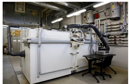
► Fig. 1: Dual Air Vented Thermal Box (DAVTB)
