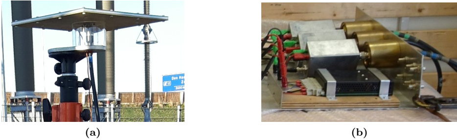
Figure 5.4: (a) Capacitive sensor design stand-alone; (b) Integrator cabinet including the passive and active integrator parts connected to a 12 bit, 4-channel digitizer.
