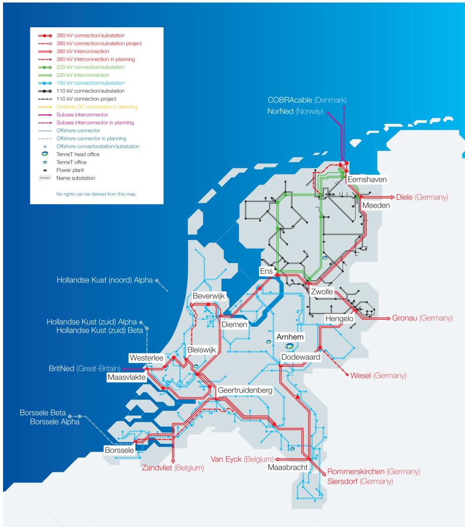
Figure 1.1: Dutch transmission network including connections and substations; red is the 380 kV, green is the 220 kV, blue is the 150 kV and black is the 110 kV network.
