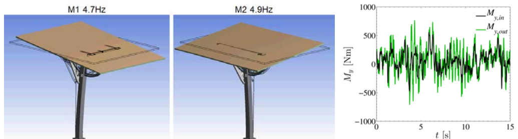
Fig. 16: Vibration behaviour of the heliostat structure at main modes (left and middle), time signals of input and output moment at the elevation axis with amplification factor 1.4 (right) (Vásquez-Arango, 2016)
