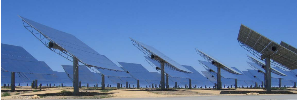
Fig. 56: Heliostats with mirror panels of 120m 2
