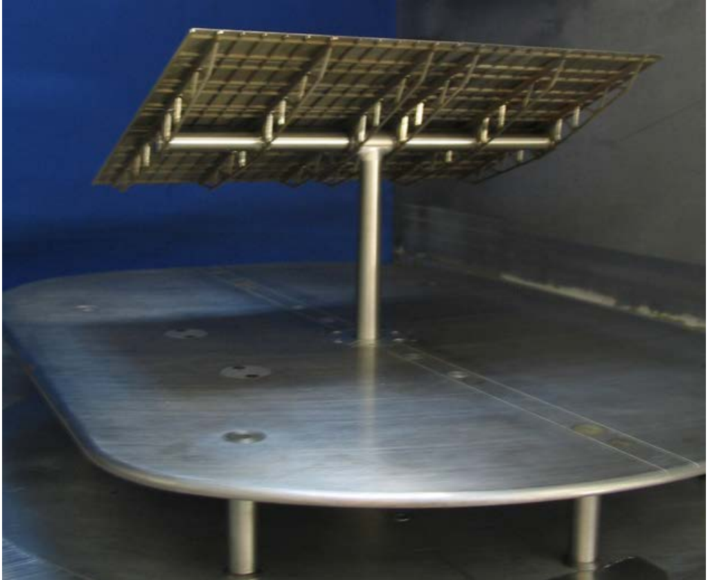
Fig. 59: Heliostat model in HDG, scale 1:50
