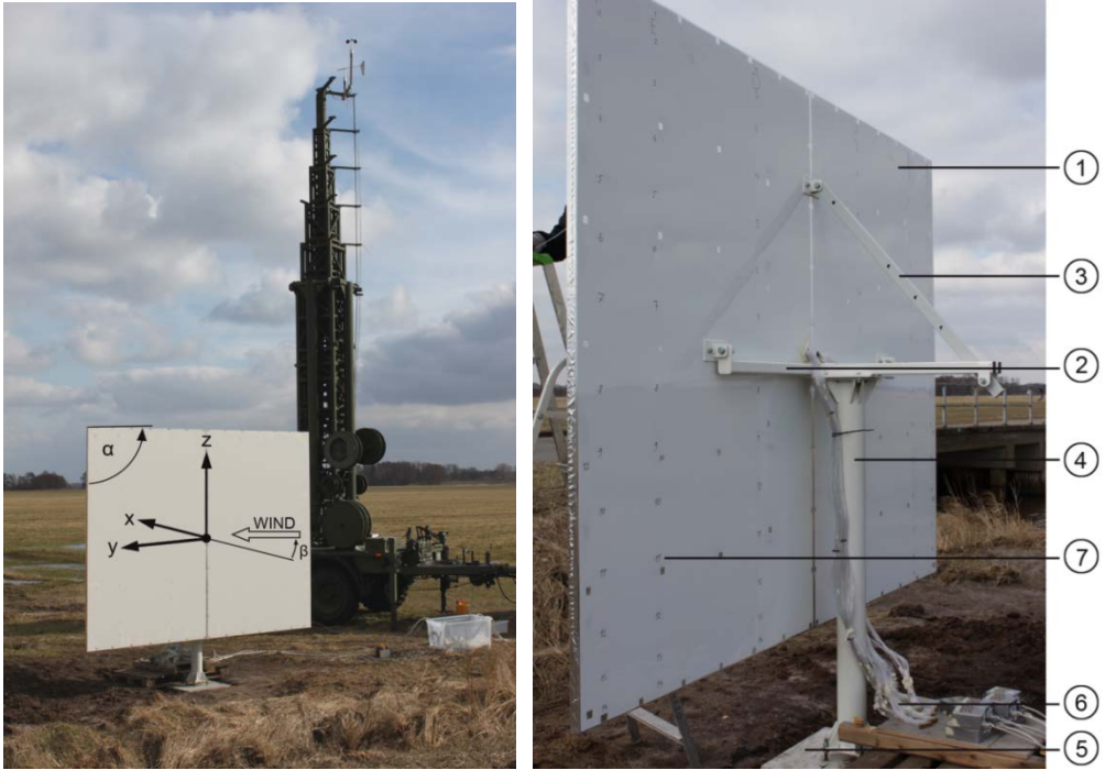
Fig. 83: left: Heliostat (size 8\text{m}^2 ) in the field, municipality Lilienthal, Germany. The chosen coordinate system according to Peterka is drawn on the facet. In the background: telescopic mast with sensors. Right: The heliostat is equipped with 84 differential pressure ports. (1) facet, (2) supporting structure, (3) elevation inclination, (4) pylon, (5) pedestal, (6) pressure tubing and instrumentation boxes, (7) pressure ports.
