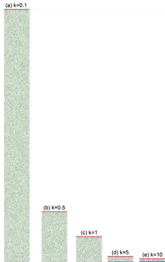
Fig. 2. Variation of the channel height for different modified Knudsen numbers in the transition regime (case H \sim ).
