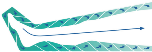
Figure 1. Schematic illustration of an inflatable leg sleeve including 12 circular air chambers. Each chamber is inflated individually to compress a section of the leg. The pressures in the individual chambers form a gradient along the leg. The highest pressure (dark green) is applied to the foot. Through external compression of the leg, a part of the peripheral blood is shifted towards the upper body.
