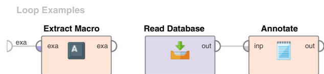
Fig. 17 RapidMiner subprocess to extract each table when connecting to a SAP database
