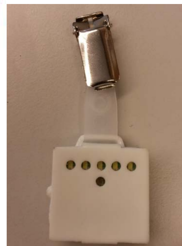
← Figure 2: A wearable light measurement device (LightLog) developed by Martin [2].
