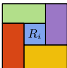
Fig. 2. A non-sliceable layout. Rectangle R_i is the center of a “windmill”.
