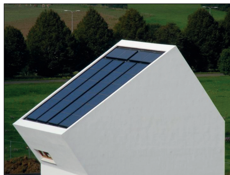
Figure 5. Photograph of the BIPV field test in of 4 portrait BIPV segments and 2 landscape solar thermal collectors at the top.
