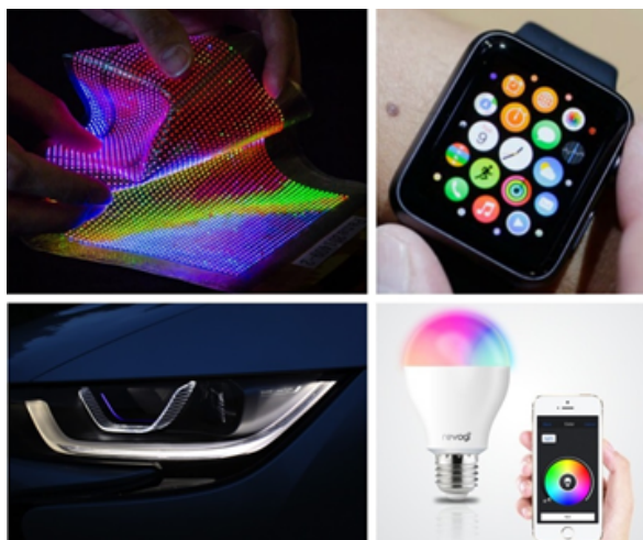
Figure 9.2: Examples of innovative LED systems. (a) A matrix of LEDs embedded in a flexible polymer for flexible LED displays. (b) Apple watch with microLED display. (c) Headlight of an Audi car, mounting a laser lighting system based on semiconductor diodes. (d) Color-tunable LED lamp, with dedicated mobile application.
