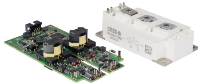
Fig. 8. Gate driver ( PT62SCMD12 ) and the chosen SiC-MOSFET ( CASI20M12BM2 ).
