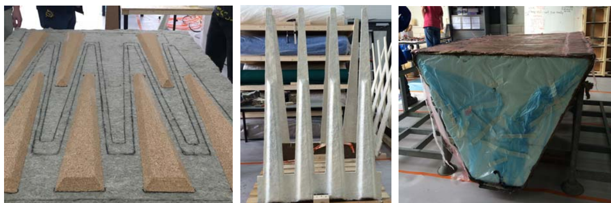
Fig. 15: Cork pieces used to reinforce the each railing element
