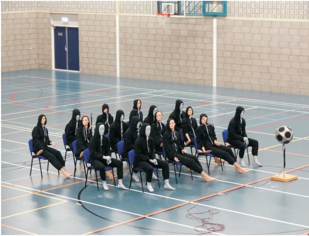
FIG. 6. (Color online) The attenuation of direct sound through a group of humans and a group of mannequins has been measured in a sports hall for validation. The picture shows the setup with the group of mannequins.
