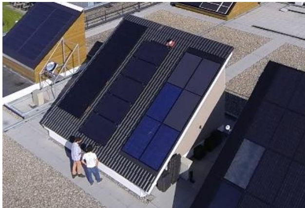
Fig. 2: Field test with three types of uncovered PVT systems on the dummy roof
