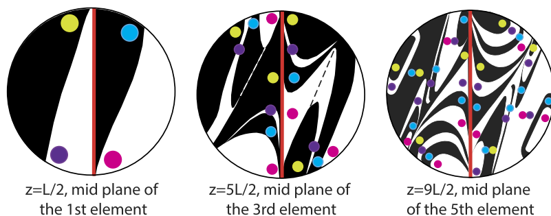
FIG. 18. Cross-sectional evolution of experimental scalar fields at 3 axial positions ( z = L/2, 5L/2, and 9L/2 ) which corresponds to the mid planes of the first elements of 1st, 2nd, and 3rd periodic segments of the Quatro mixer. The circles in color (yellow, pink, blue, and purple) are used to tag the evolving regions for a better understanding of the scalar evolution. Right half of the rightmost image is enhanced by using anti-symmetry.
