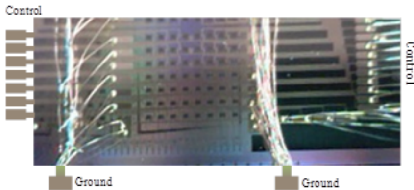
Figure 2.5: Photograph of assembled circuit. Wire bonds leading to the left and right of the image are control lines. Wire bonds leading to the bottom edge are the common ground lines.
