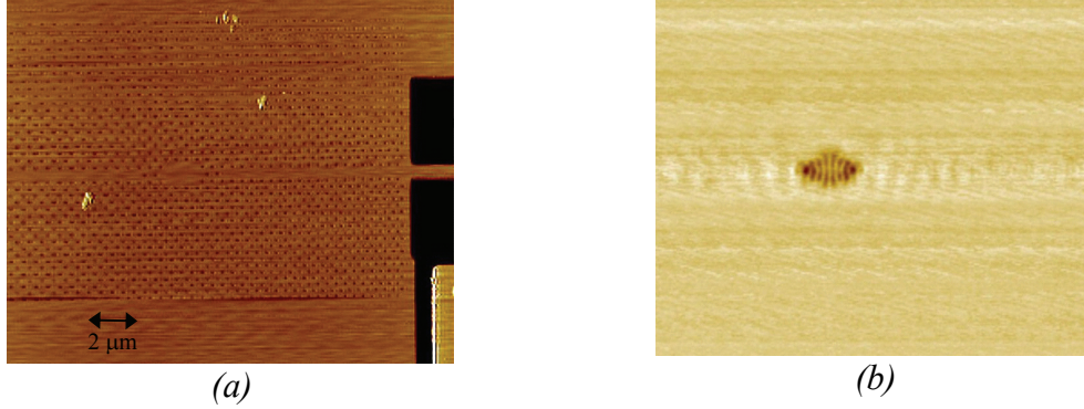
Fig. 3. (a) AFM height data, obtained by scanning a \text{Si}_3\text{N}_4 tip over the PhC structure in contact mode. (b) While scanning, the transmitted power was monitored and graphically visualized in a 2D image.
