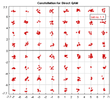
a) Constellation for Direct QAM
