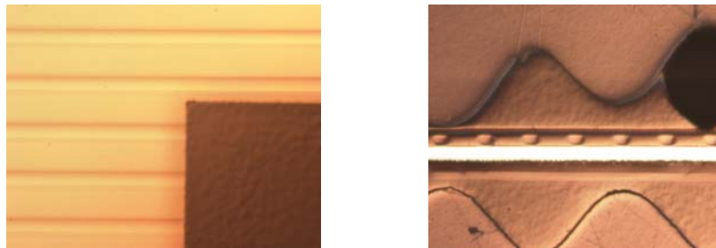
Figure 4: Embedded 5x5 cm 2 dummy chip and waveguides in Ormocer® material. left : Top view right : Cross section.
