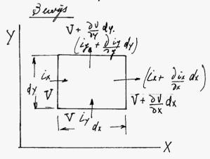
In X pichting geldl:  $\Delta V_x = I_x R_x$   $\Delta V = \text{Spannings Nerbehil}$  I = Istale stroom k = weesstand. l = Specifieke weerstand. l wordt constant verondusteld.
