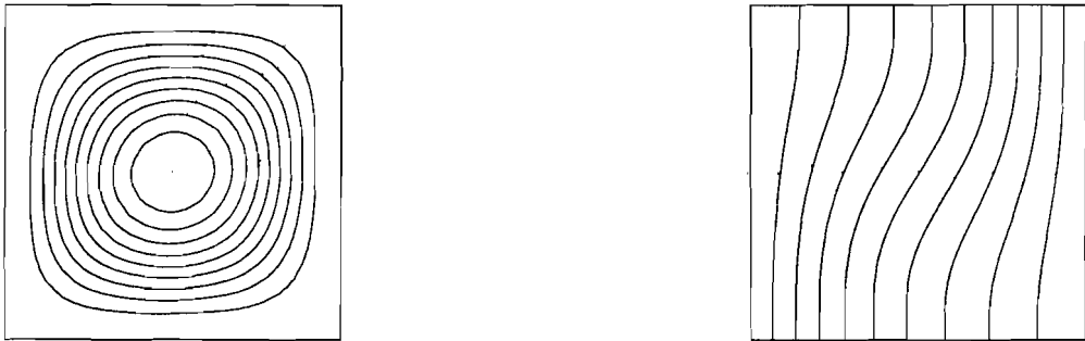
Figure 4.4: Streamlines (left) and isotherms (right) for the buoyancy-driven flow in an enclosed cavity at R = 10^3 . Modified pressure correction/operator splitting scheme using 4 \times 4 elements of degree N = 8 .
