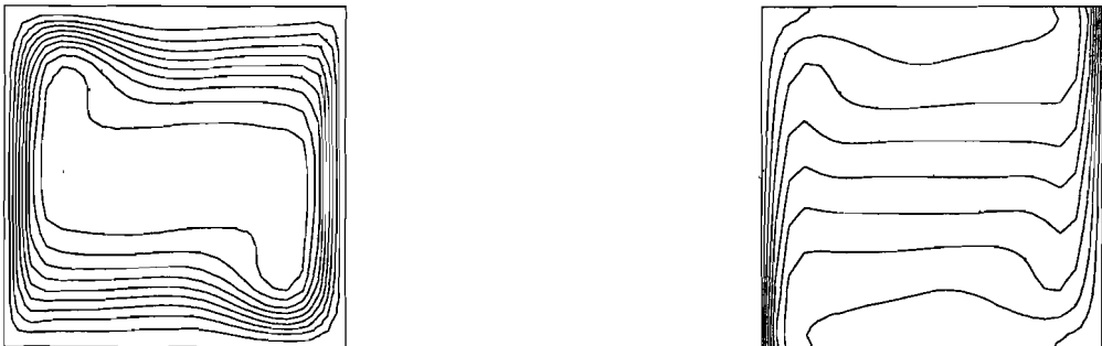
Figure 4.5: Streamlines (left) and isotherms (right) for the buoyancy-driven flow in an enclosed cavity at R = 10^6 . Modified pressure correction/operator splitting scheme using 4 \times 4 elements of degree N = 8 .
