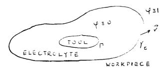
an electrolytic circuit. The current flows in the electrolytic solution under the action of a potential difference between the electrodes and causes dissolution of the anode surface which allows for micrometric machining of the workpiece.
