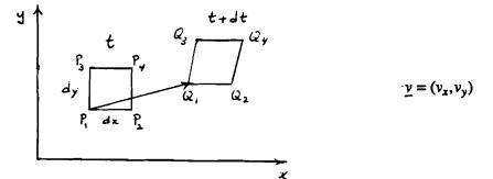
At time t we have  $P_1 = (x, y)$ ,  $P_2 = (x + dx, y)$ ,  $P_3 = (x, y + dy) P_4 = (x + dx, y + dy)$ .
