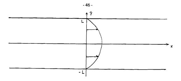
For the velocity field we take  $\vec{v}(x,y) = (v(x,y), 0)$ , i.e. a Poiseuille flow. Adding no-slip conditions at the boundary, i.e. v(x,L) = v(x, -L) = 0 we obtain the solution
