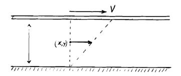
Given two plates at y = 0 and y = d, the plate at y = 0 remains at rest while the other plate at y = d move in the x-direction with a constant velocity V. Between these plates there is a flow of a Newtonian fluid with viscosity  $\eta$  and with a homogeneous mass density  $\rho_0$ .
