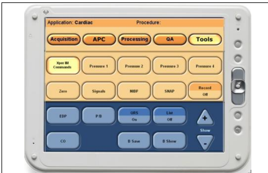
Figure 9 – The touch screen module used in the operating room
