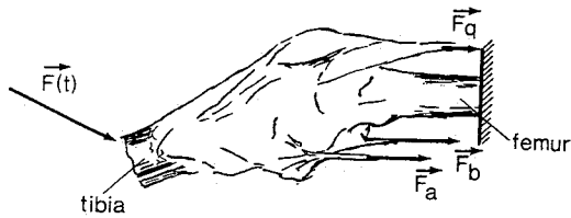
Fig. 1 Schematic view of a joint specimen clamped at the femur and loaded with a dynamic force F(t) at the tibia while static tensile forces F_a , F_b and F_q are acting at the tendinous muscle attachments
