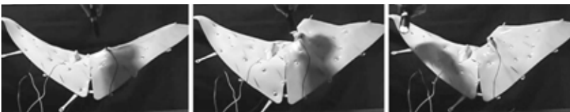
Fig. 13. Morphological transformation of the triangular modules of Blind responding to direct light for optimal performance.
