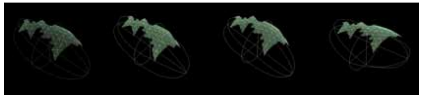
Fig. 9. Blind in the form of a semi-ellipsoid canopy performed morphological transformation for optimal sunlight manipulation.
