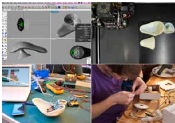
Fig. 8. Making the final prototype, using McNeel's Rhino 3D modelling software, 3D printing, an Arduino microcontroller board and Cycling74's MaxMSP programming environment.
