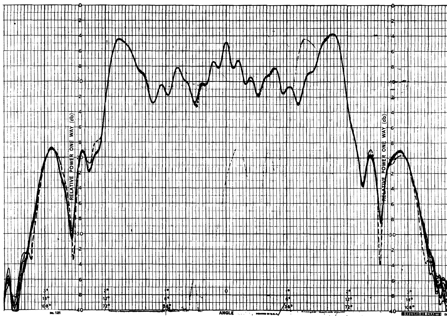
Fig. 6: Highly-shaped beam antenna, LHCP, f = 12.05 GHz, feed supports in horizontal position, azimuth pattern.
