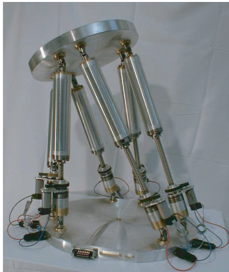
Figure 6.4: Example of a hexapod system with lead-screws
