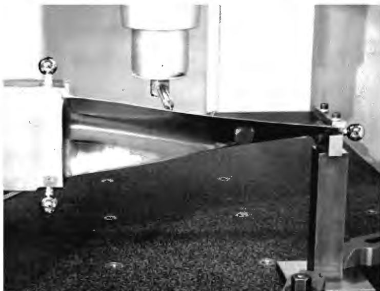
figure 1: The turbine blade being measured in one of the different workpiece orientations, to estimate the uncertainty contribution from the geometrical errors of the CMM.
