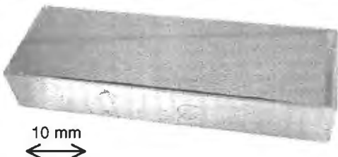
figure 1: 10 nm Pt-layer as thickness standard for X-ray facilities on a fused silica
