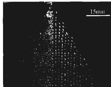
figure 5: Injected spray pattern and velocity diagram
