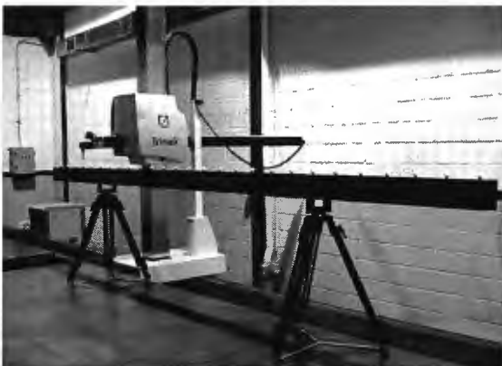
figure 1: 4m ball bar of carbon fibres on a CMM
