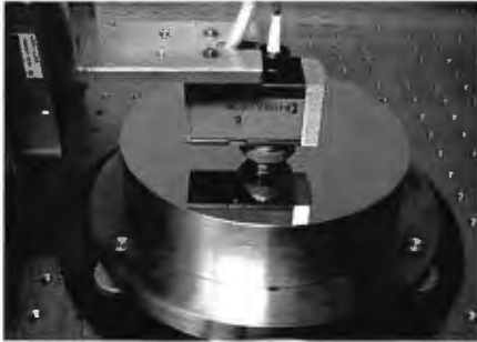
figure 1: The small interferometer used as curvature sensor is guided along a diamond-turned aspherical profile on a flat substrate.
