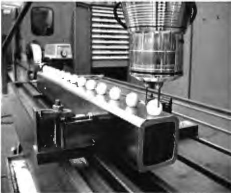
figure 5: self centring probe on a machine tool while measuring a ball bar
