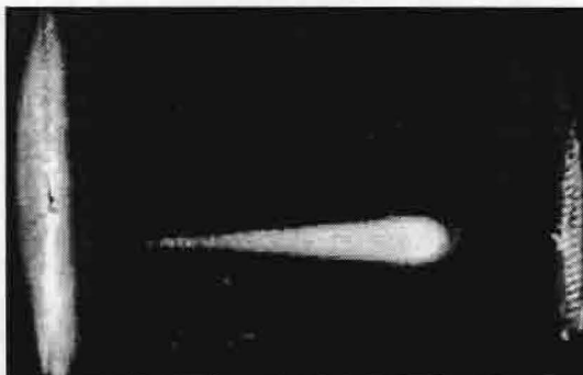
Fig. 1: Cloud track picture of a single avalanche, cathode at the left (by H. Raether, [5]).
