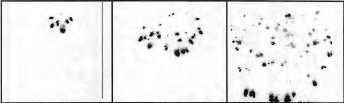
Fig. 3: Pictures of streamer propagation in a point-to-plate gap using a 0.8 ns intensifier gate, real size per frame \sim 3 \times 3 \text{ cm}^2 (picture by A.H.F.M. Baede)
