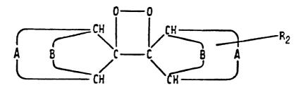
in which A and B represent alkylene radicals, which alkylene radicals may be attached to each other via an alkylene radical C, and  $R_2$  represents chloro, bromo, or iodo, a hydroxy group, an optionally substituted alkoxy, cycloalkoxy or acyloxy group, or an amino, acylamino, thiocyanato or isocyanato group, the substituent  $R_2$  to a substituent  $R_1$  within the meanings for  $R_1$  given in claim 1.
