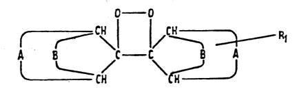
in which A and B represent alkylene radicals, which alkylene radicals may be attached to each other via an alkylene radical C and  $R_1$  represents chloro, bromo or iodo, a hydroxy group, an optionally substituted alkoxy, cycloalkoxy or acyloxy group, or an amino, acylamino, isothiocyanato or isocyanato group, with the proviso that in the case of a 4-eq.- $R_1$ -2,2'-epidioxy-2,2'-adamantyl adamantane  $R_1$  cannot be chloro or hydroxy.
