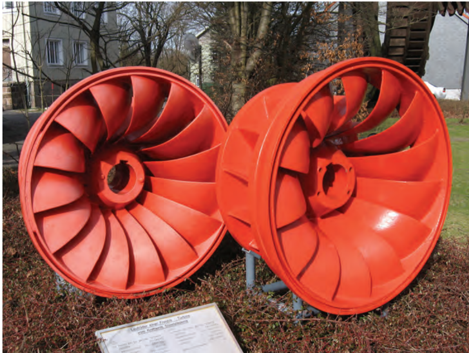
Figure 68: Francis turbine (Wikipedia)
