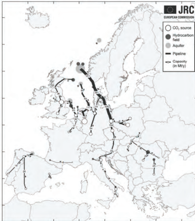
Figure 32: CO 2 pipeline network in 2050, assuming joint international optimization. Total amount of CO 2 captured and stored: 1145 Mt/y. (Ref: Fig 5.1 of [Morbee, 2012])
