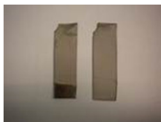
Figure 5.1. A brown layer could clearly be observed on the cathode (left electrode)
