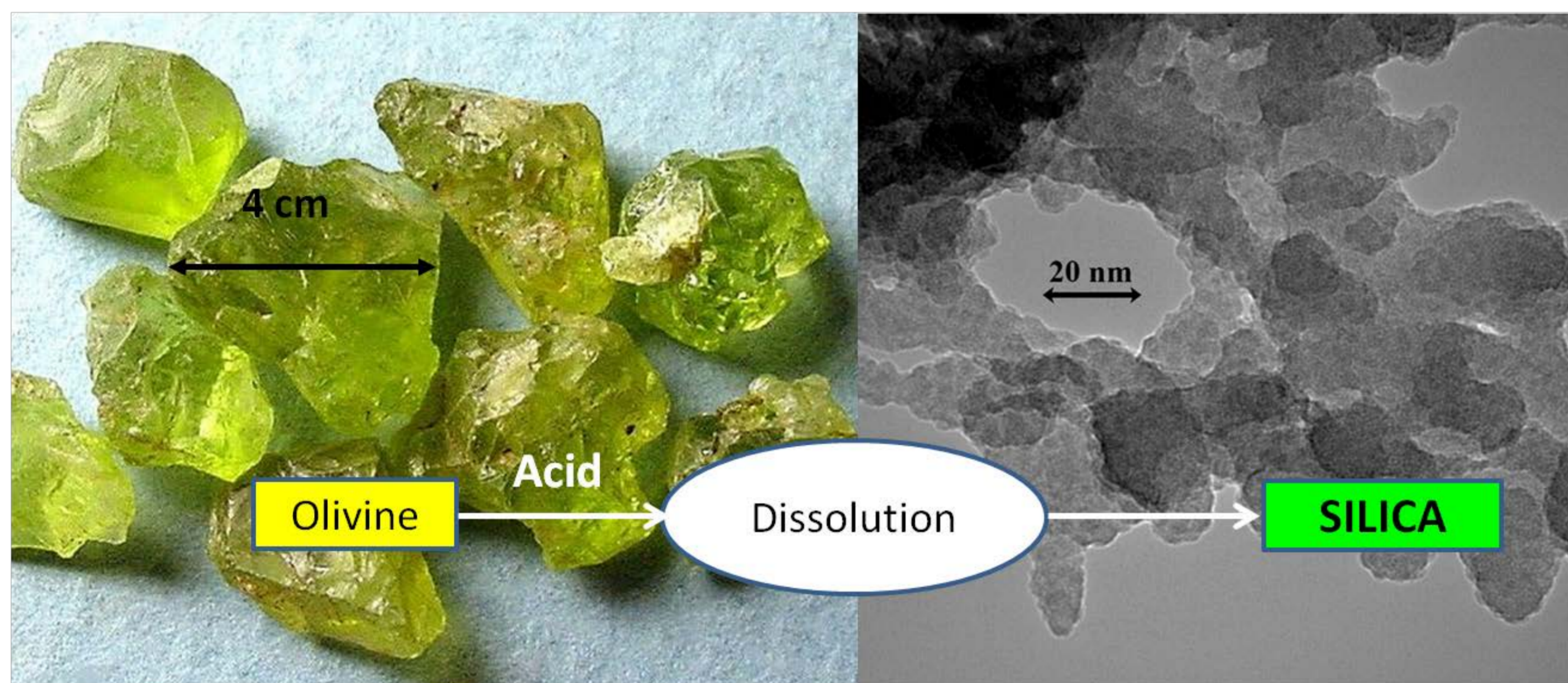
Featured article and cover of the Chemical Engineering Journal [2]: The properties of amorphous nano-silica synthesized by the dissolution of olivine.
