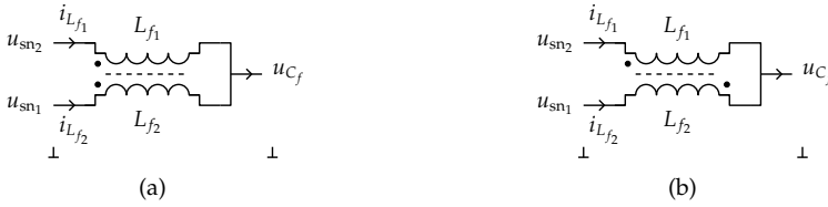
Figure 5.3: Coupled DB filter inductor with (a) positive coupling, and (b) negative coupling.
