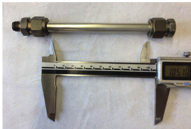
Fig. 4 – Pd membrane (E80 – Pd–Ag membrane, thickness 4.5 micron) before and after connecting to the Swagelok® connectors.
