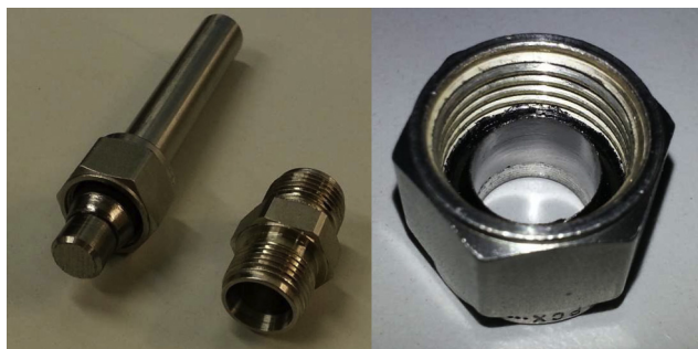
Fig. 3 – Left: 316L dummy rod with graphite ferrule and Right: connector with pre-treated ferrule (shiny inner surface).
