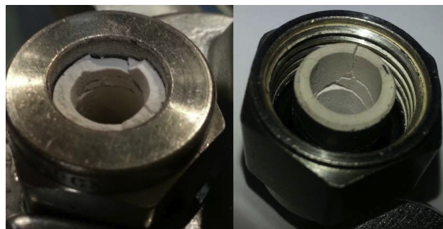
Fig. 5 – Broken Membrane after applying 14 Nm.
