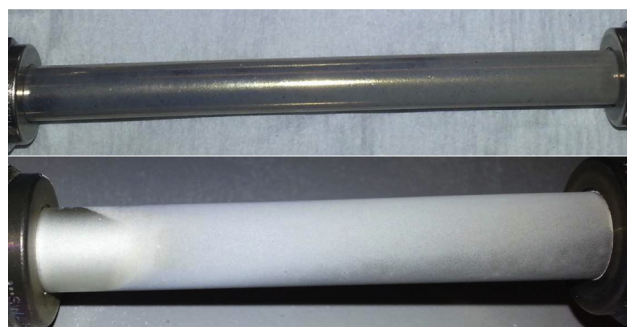
Fig. 17 – E54 membrane before and after fluidization tests with bed #1.
