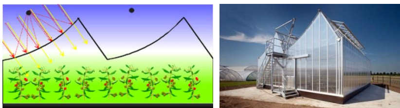
Figure 2.16 Schematic description of application of NIR-reflecting film (left) (Sonneveld, Swinkels, Bot, et al. 2010) and Mock-up model of ELKAS (right) (Sonneveld, Swinkels, Campen, et al. 2010)
