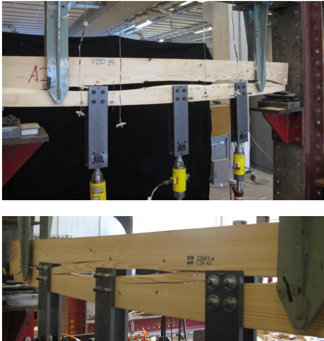
Figure 8: Test beam after failure with three connections
