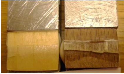
Figure 15: Typical EPX shear test specimen after testing
