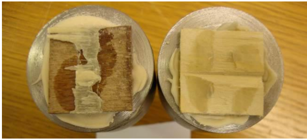
Figure 16: Typical tensile test specimen after testing
