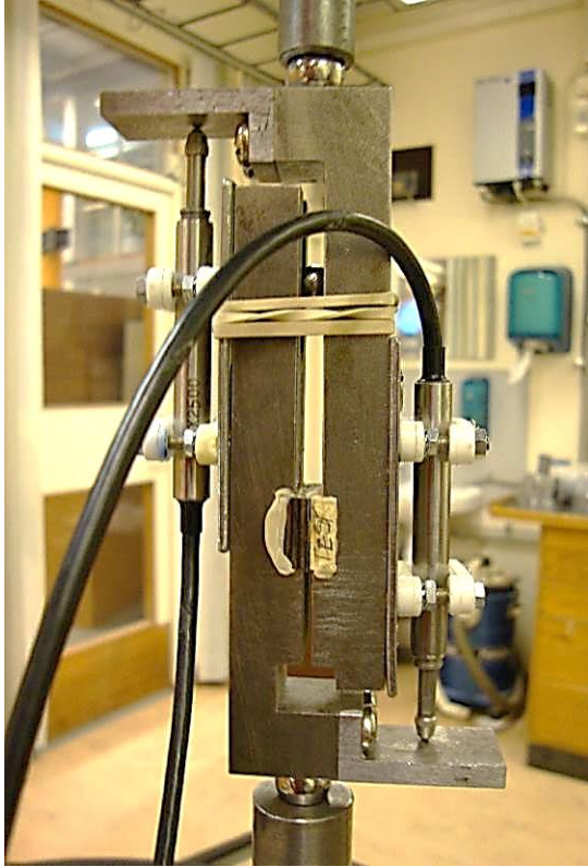
Figure 4: Bond line shear test
