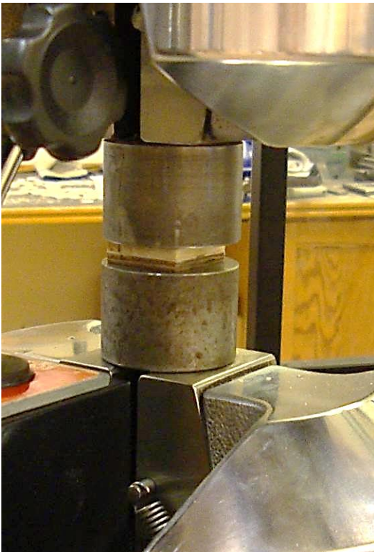
Figure 5: Bond line tension test
