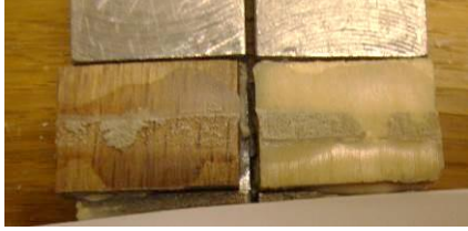
Figure 14: Typical PU shear test specimen after testing
