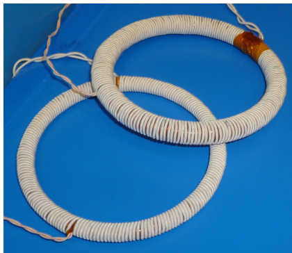
Figure B.2: Example of a fully wound ring sample.
