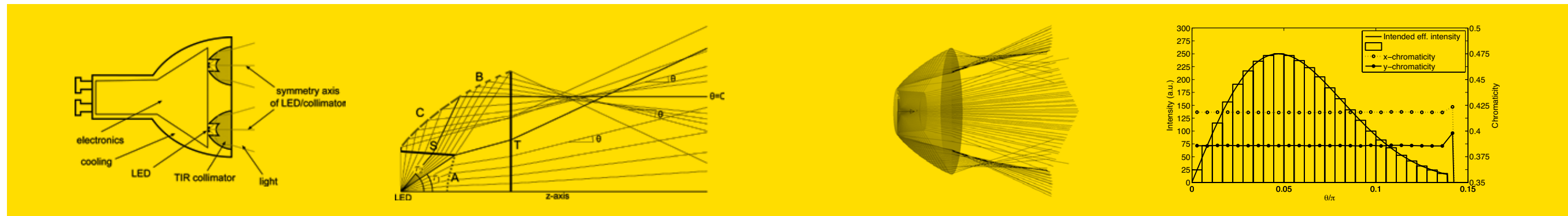
Figure 1: Schematic drawing of an LED-based halogen spot replacement.
