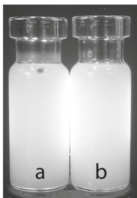
Figure 5.15 left: SDD1 before (a) and after (b) centrifugation at increased gravity ranging from 7 \cdot 10^5 to 1.7 \cdot 10^6 m \cdot s^{-2} . right: TGA of SDD1 ( m_0 = 39 mg). After reaching a temperature of 120 °C the temperature was kept constant at this value for 60 minutes to allow for evaporation of water. The heating rate was 10 °C min^{-1} . The inset shows the conventional residual weight vs. temperature plot starting at 120 °C ( i.e. after removal of the continuous water phase).
