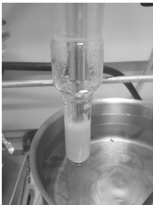
Figure 5.3 left: Reactor setup used for the synthesis of poly(hydroxy urethane) resins and for producing dispersions. A magnetically coupled stirring setup is fitted to ensure a closed system. Properties of the double helical ribbon impeller: diameter 13 mm, ribbon width 2 mm, shaft diameter 3 mm, length 30 mm, pitch 1 rotation/10 mm, stainless steel. right: SAH1 during dispersing.
