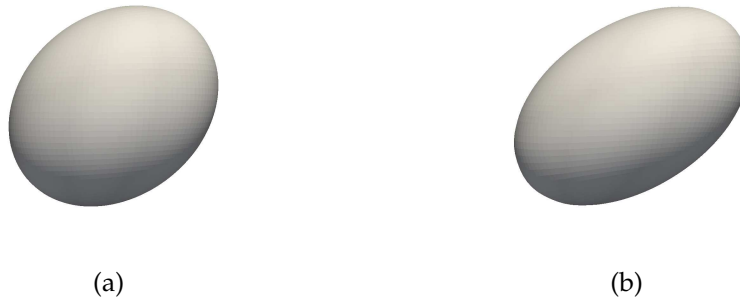
Figure 6.21 Stable drop shape using the hybrid geometry with 288 elements for (a) Ca = 0.1 (b) Ca = 0.2 .
