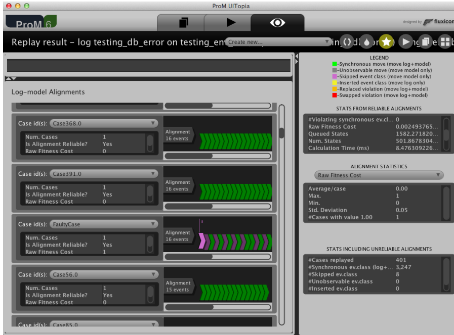
Figure 103: Visualizing the alignments of Fail(D) to env(mp_1(max_1(D))) in ProM. The alignment \gamma_6 from Ex. 180 is depicted in the middle of the screen: All non-silent model moves are shown in violet, and all synchronous moves are shown in green.
