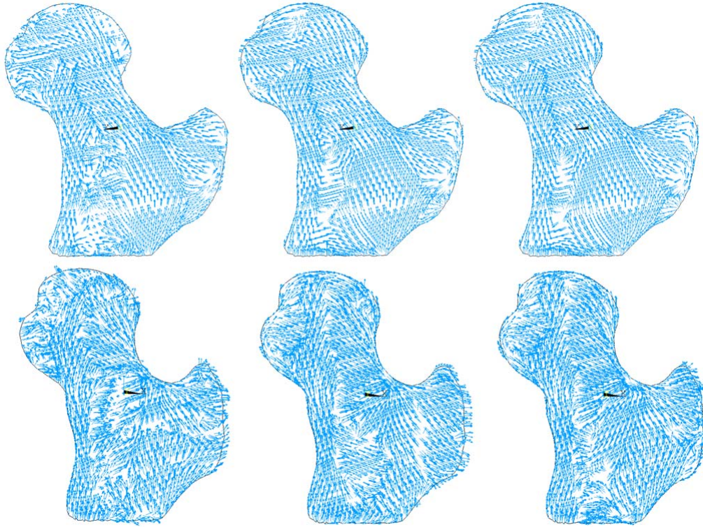
Figure 9. Maximum principal stress vector plots for micro-FE (left), orthotropic (middle) and isotropic (right) models for the healthy femur (top) and osteoporotic one (bottom).
